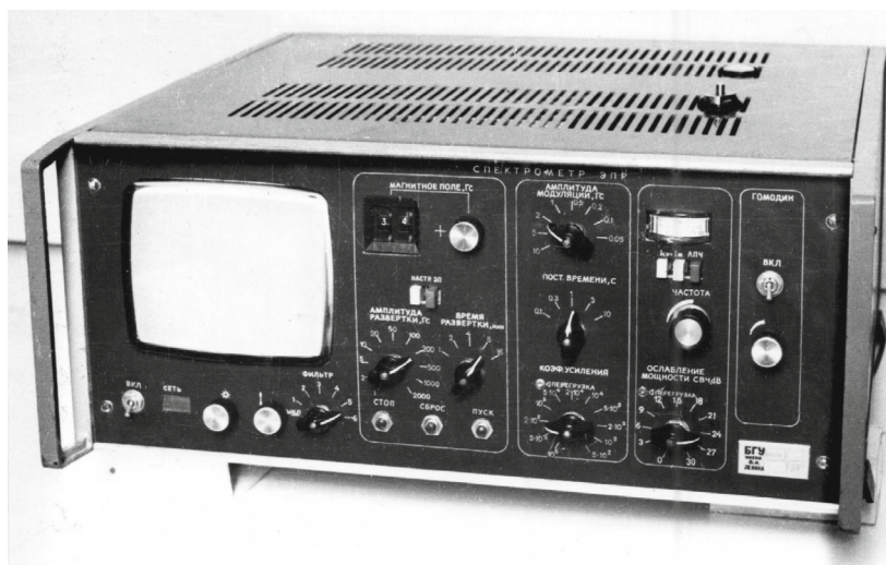
Fig. 12. Specialized compact EPR spectrometer constructed by V. N. Linev's team at BSU early in the 1980s. Source: personal archive of V. N. Linev.
