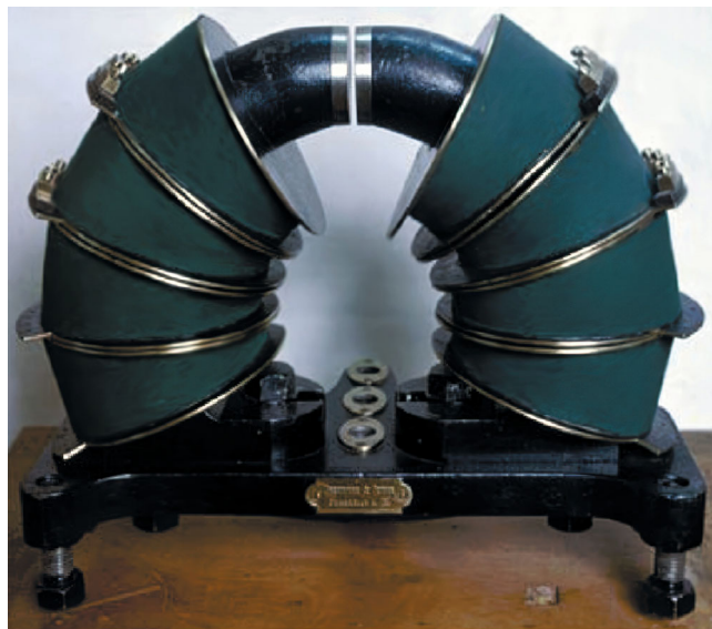
Fig. 4. The du Bois-Reymond-type electromagnet, employed by E. K. Zavoisky, S. A. Altshuler and B. M. Kozyrev in their experiments in late 1930s. Kazan, E. K. Zavoisky Laboratory Museum. Source: I. I. Silkin's personal archive.
