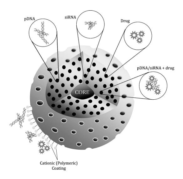
Schematic representation of the general features of MSNs for nucleic acid and drug delivery. The surface is typically covered with cationic polymers or other molecules containing positively charged terminal functional groups to complex the nucleic acid. The pores of MSNs can hold nucleic acids, drugs, or a combination of both
